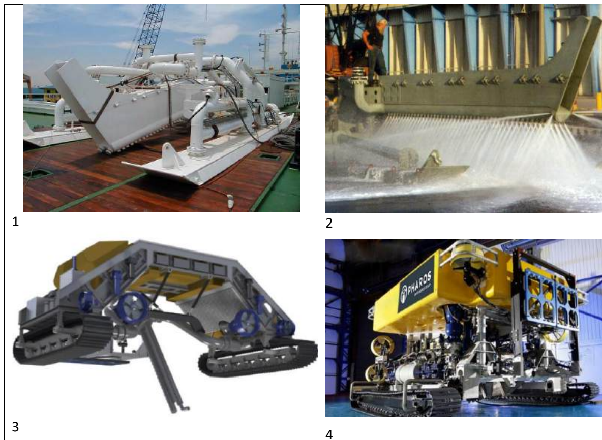
Figure 3.5. Examples of plough (1, 2) and crawler (3, 4) vehicles used for the construction as part of the water jetting and mechanical trenching technologies [Source: eta-ltd.com, ctoffshore.dgweb.dk, pharosoffshoregroup.com]
