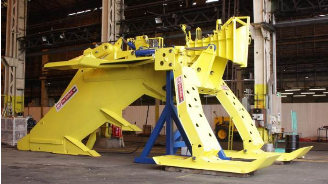
Figure 3.4. Example of a subsea cable plough [source: royalihc.com]
